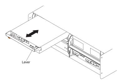
Figure 77. Removing a controller from the DS5020
